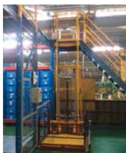
Single Mast Lift for Mezzanine
