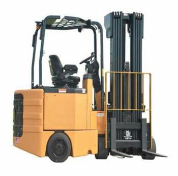
The Bendi Electric Narrow Aisle trucks are available with three-stage masts, with lift heights up to 12.5M. Four-stage masts also are available on all 4-wheel models for lift heights up to 7.92M, giving the Bendi high stacking ability, while allowing the low mast height necessary to work in highway trailers or travel through low doorways.
